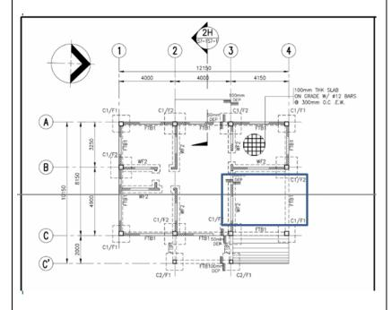
The slab is 150mm thk, with Ø12 @ 250 mm o.c. e.w.
