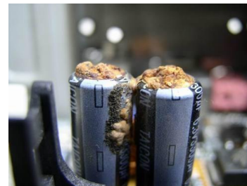
"Liquid explode" of traditional capacitor, an example
